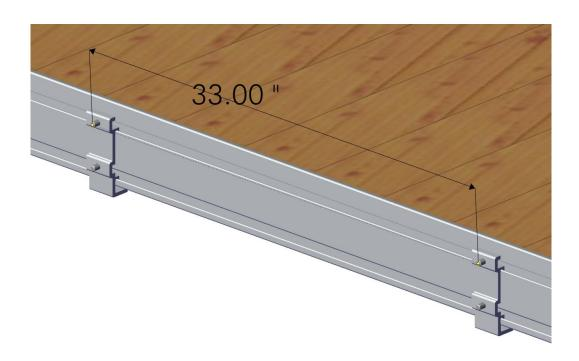
STEP 3 INSERT (2)  $3/8-16 \times 1''$  BOLTS INTO BOTTOM OF EACH QUICK ATTACH BRACKET. TORQUE TO 5 FT-LBS MAXIMUM.
